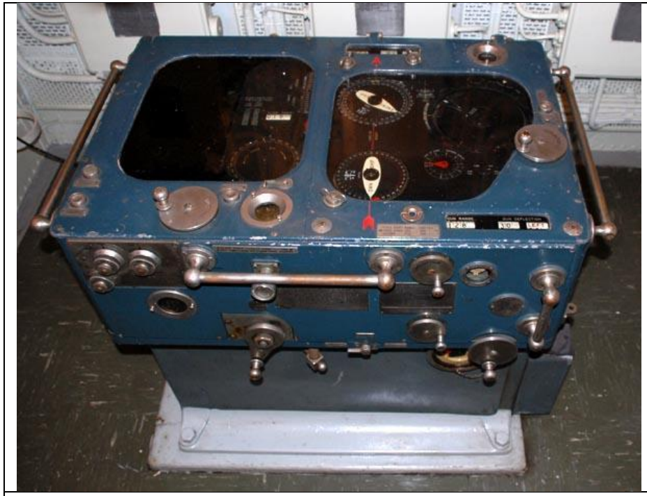
The Fire control clock in the Transmitting Station.
